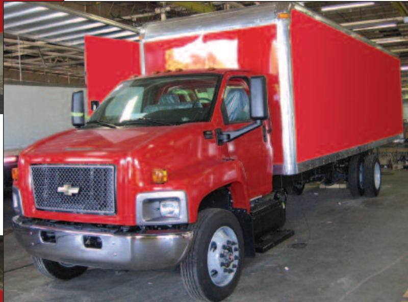
All aluminum rivetless body with diamond treadplate skirting.
